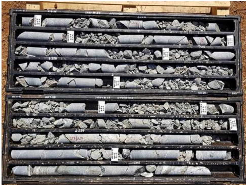
Figure 3 An example of broken drill core from KPDD002
